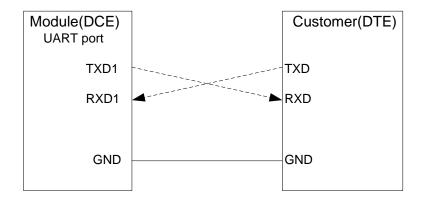
Figure 10: Connection of serial interfaces
