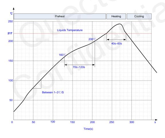
Figure 21: Ramp-soak-spike-reflow of Furnace Temperature
