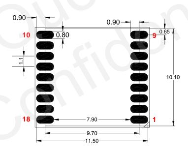
Figure 18: Footprint of Recommendation (Unit: mm)
