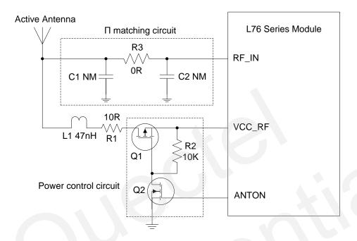
Figure 13: Reference Design for Active Antenna with ANTON
