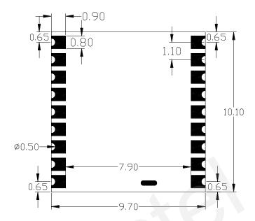
Figure 17: Bottom Dimension (Unit: mm)
