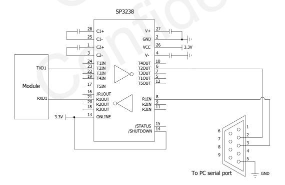
Figure 11: RS-232 Level Shift Circuit
