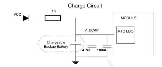
Figure 5: Reference Charging Circuit for Chargeable Battery
