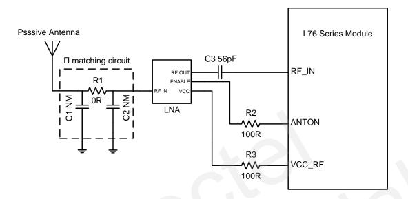
Figure 15: Reference Design for Passive Antenna with LNA
