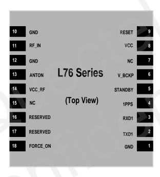
Figure 2: Pin Assignment
