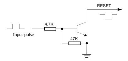
Figure 8: Reference Reset Circuit using OC Circuit
