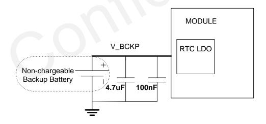
Figure 4: RTC Supply from Non-chargeable Battery
