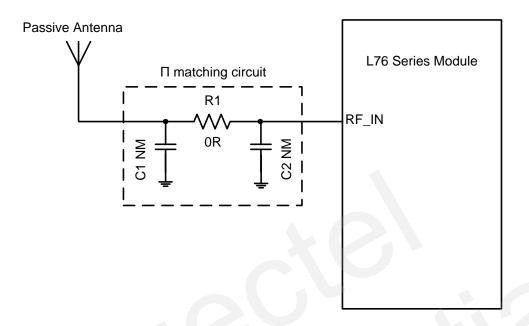
Figure 14: Reference Design with Passive Antenna
