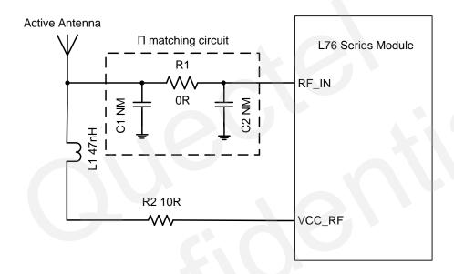
Figure 12: Reference Design with Active Antenna
