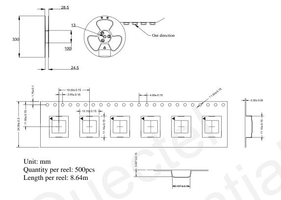
Figure 22: Tape and Reel Specification
