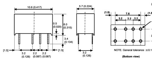
Tolerance of lead pitch is  $\pm 0.15$ mm (0.006inch) Other tolerances  $\pm 0.3$ mm (0.012inch)
