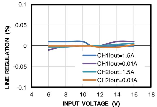
**Line Regulation vs. Input Voltage**
