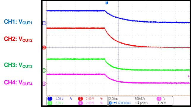
$V_{IN}$  On with Load
