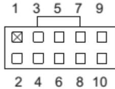
Figure 1: 10-Pin Ribbon Cable Bottom View
