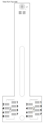
Figure 10: Connector RD Pinout Type 1
