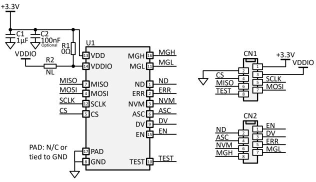
Figure 23: Schematic RD/LT Type 3
