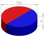
Figure 39: Cylinder Magnet, Diametrically Magnetized
