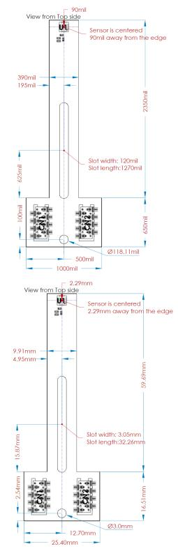
Figure 27: Mechanical Drawing LT Type 3 mil = 0.001in = 0.0254mm
