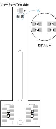
Figure 6: Assembly View RD Type 1
