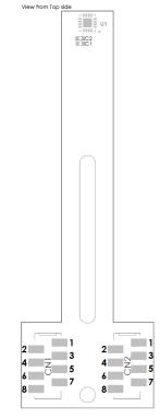
Figure 19: Connector RD Pinout Type 2
