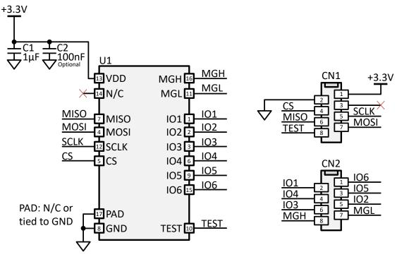
Figure 14: Schematic RD/LT Type 2
