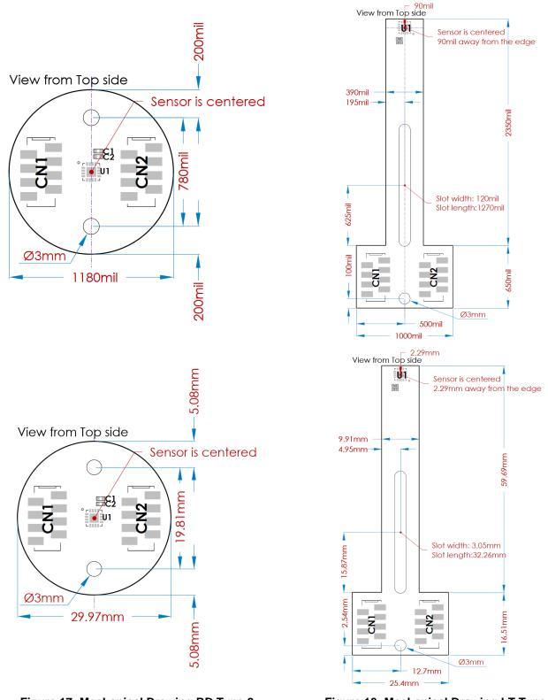
Figure 17: Mechanical Drawing RD Type 2
