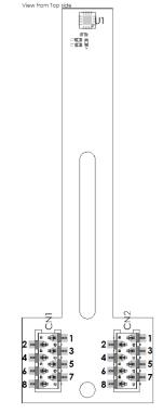
Figure 28: Connector RD Pinout Type 3
