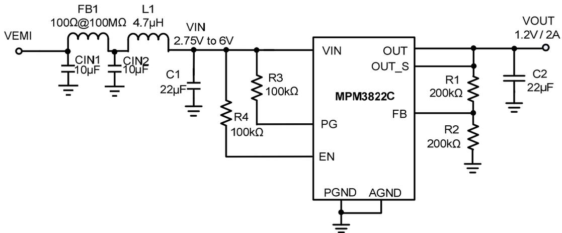
**Figure 5: EMI Test Circuits for the MPM3822C**
