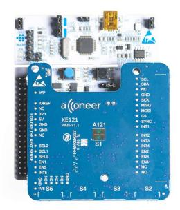
Picture 6. XE121 connected to an STM Nucleo Development Board.
