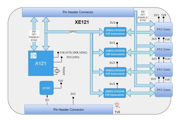
Picture 1. The blockdiagram of XE121.
