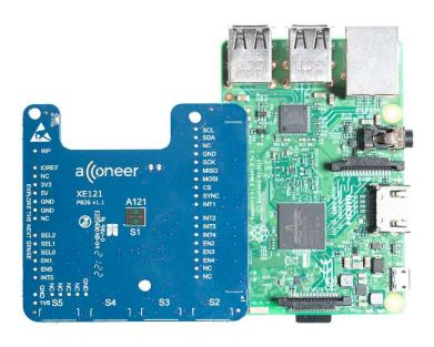
Picture 5. XE121 connected to Raspberry Pi.
