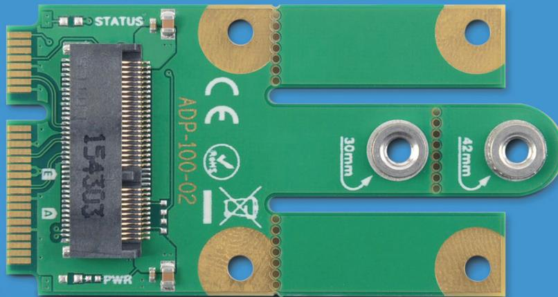
It is an adapter for BLACK bean and other M.2 form factor radio modules that fit into the standard mini PCI express slot. The adapter supports PCIe and USB2.0 system bus interfaces. It also allows connecting mini PCI express modules such as LTE, 3G, GPS, and Bluetooth. No drivers are necessary for this M.2 to mini PCI express card adapter.
