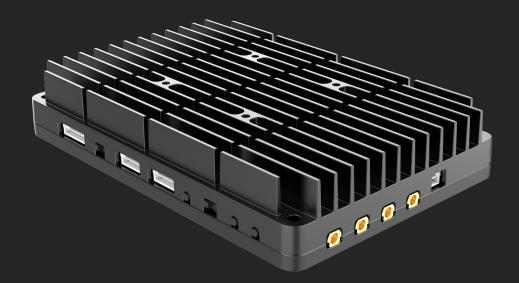
Robonode is a highly efficient, low-latency, long-range data radio optimized for drones and robotic missions. Designed for critical communication in unmanned systems, this radio features Wi-Fi broadcasting with Forward Error Correction (FEC), fast frequency shifting, narrow channels, and additional capabilities to ensure stable and reliable connectivity in demanding environments.
