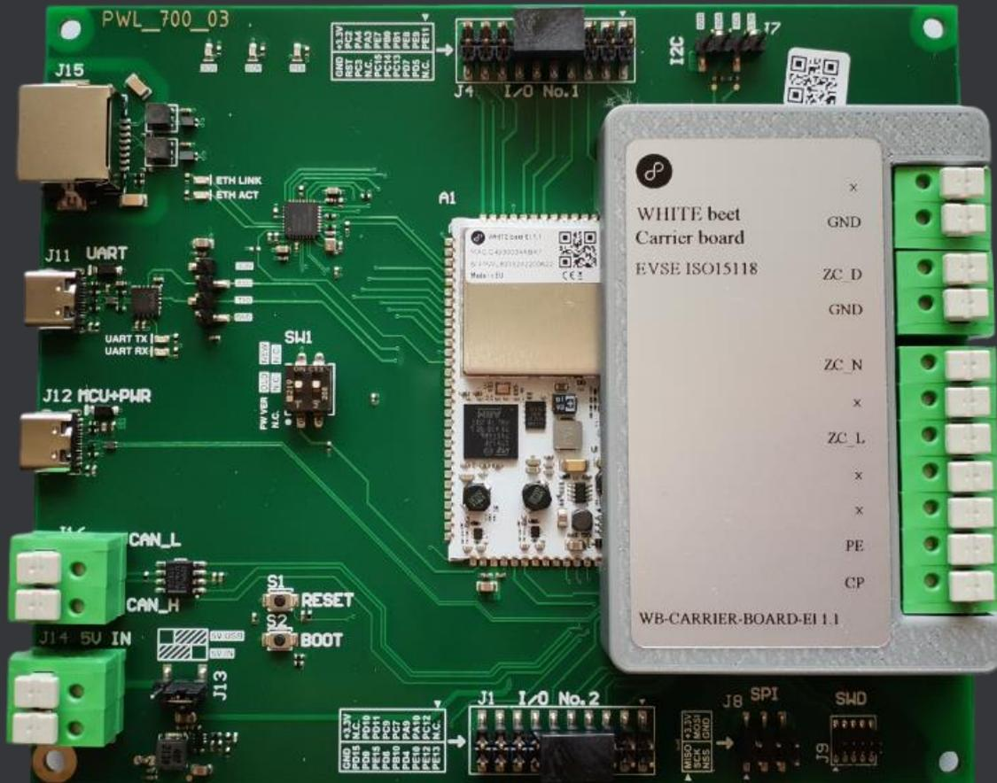
**WB-CARRIER-BOARD 1.1** is an evaluation and development board for WHITE-BEET 1.1 modules. It contains WHITE-BEET 1.1 module populated on the carrier board and protected with a plastic cover.
