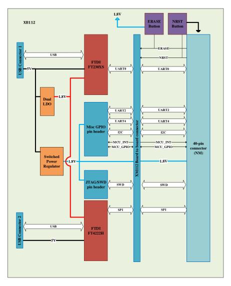
Figure 1 The EVK block diagram.
