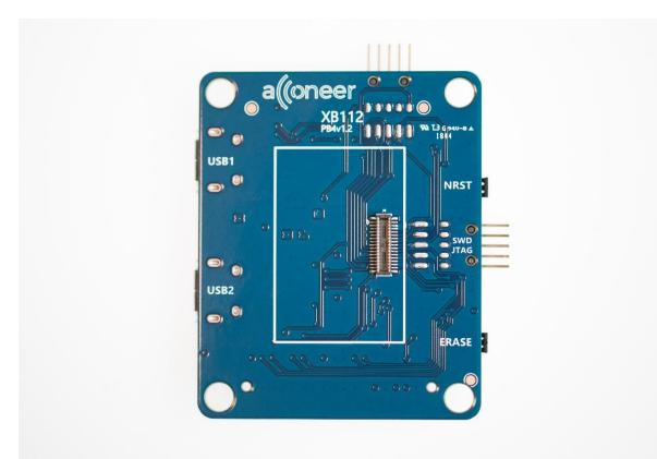
Picture 1 shows the XB112 connector board, front side.
