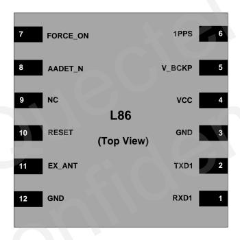
Figure 2: Pin Assignment
