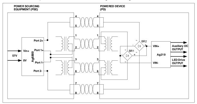
Figure 3: Typical System Diagram
