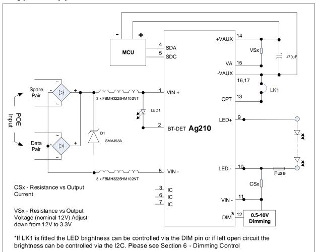
**Figure 11: Typical Connection Diagram**
