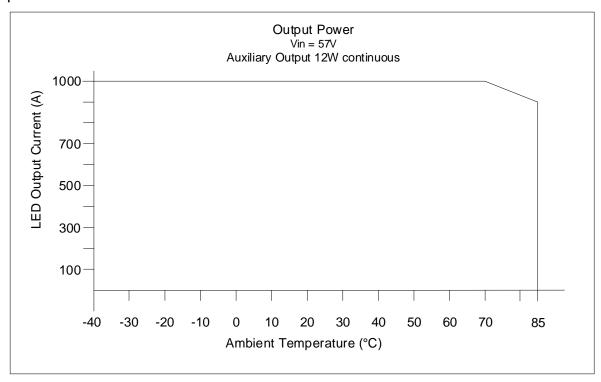
Figure 10: Operating temperature
