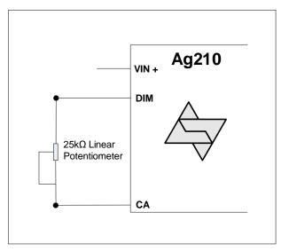
Figure 9: Resistive Dimming Control
