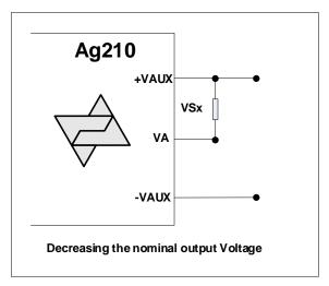
**Figure 5: Output Voltage Adjustment**
