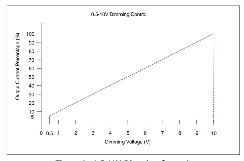
Figure 8: 0.5-10V Dimming Control
