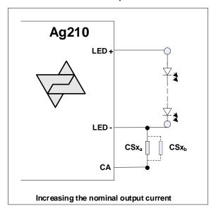
**Figure 4: Constant Output Current Adjustment**
