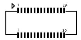
Figure 2.2. XM122 J2 connector footprint.
