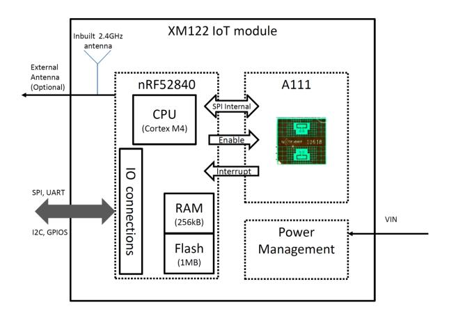
Figure 2.1. XM122 block diagram.
