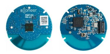
Figure 1. XM122 Top view (left) and XM122 bottom view (right).
