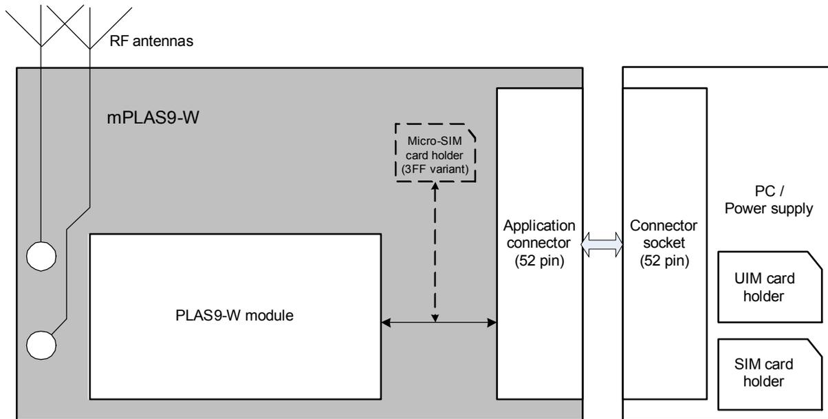
Figure 3: LTE Modem Card mPLAS9-W system overview
