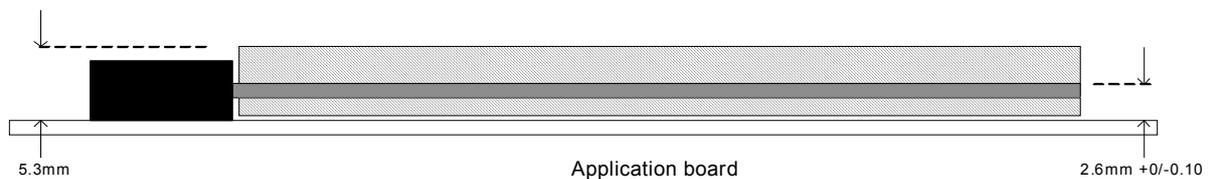
Figure 4: LTE Modem Card mPLAS9-W mechanical dimensions (height)
