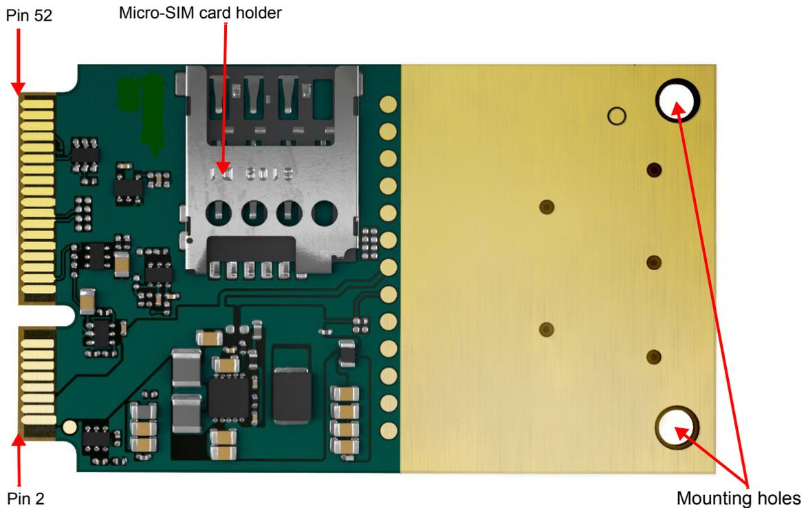
Figure 2: LTE Modem Card mPLAS9-W bottom view
