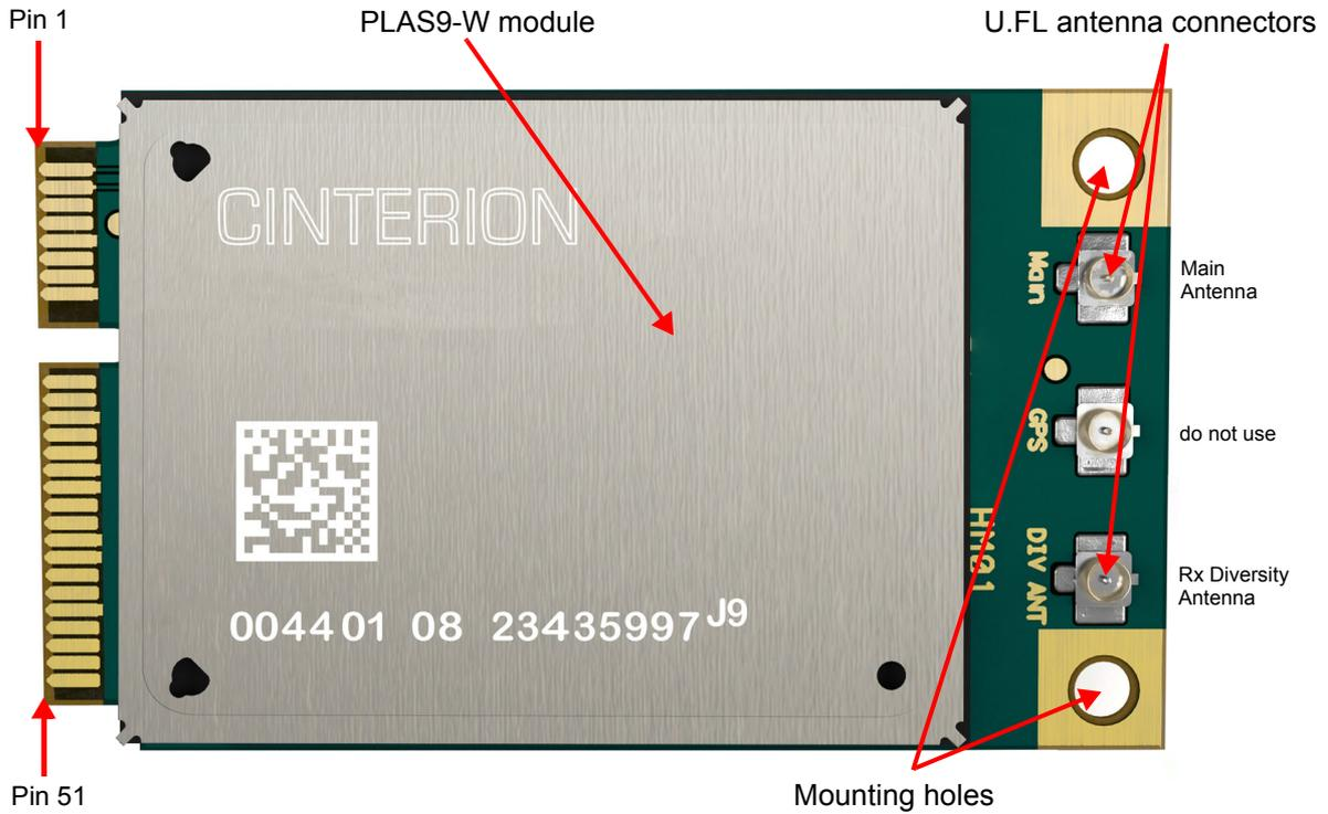
Figure 1: LTE Modem Card mPLAS9-W top view
