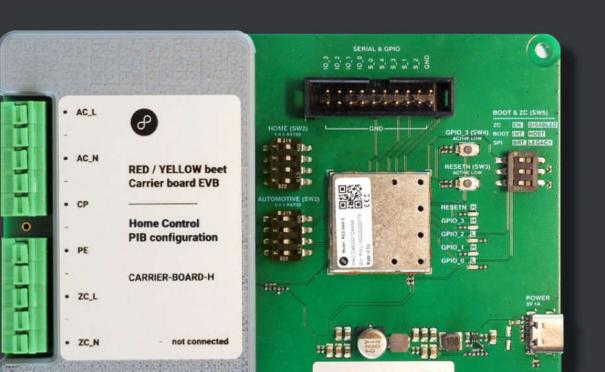
Carrier board allows testing and evaluation of RED and YELLOW beet modules in all applications starting from e-Mobility (EVSE and PEV) to other enterprise and home applications requiring long-range communication like smart grid, smart meter, IoT, home control and etc.
